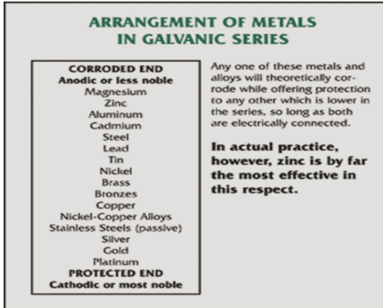
Figure 1. Summary of the “electromotive series of metals” address on corrosion.
